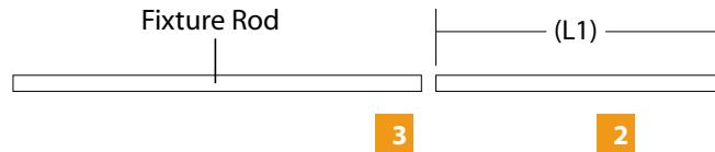
**NOTE:** To avoid interference while relamping do not cut the fixture rods (L1) more than 24" inches.
